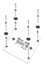
Step 2: Mount the brackets on the USG and screw it tight.
