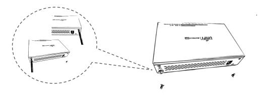
Step 2: Mount the brackets on the US-8-60W and screw it tight.
